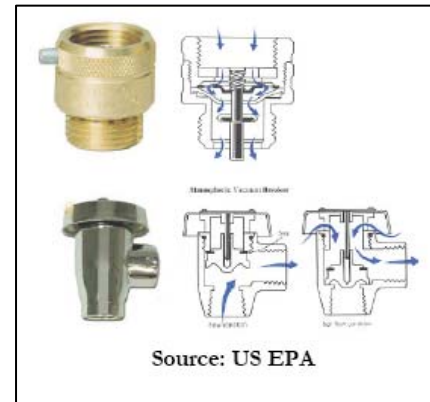
Figure 11 – Atmospheric Vacuum Breaker
